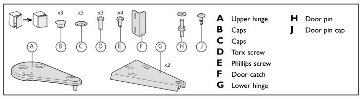
This allows you to change the direction in which the door opens. Follow the instructions below (example for changing a right-hand door into a left-
