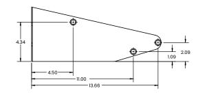
ROD POSITIONS, DISPLAY BRACKET 1 REMOVED FOR CLARITY
