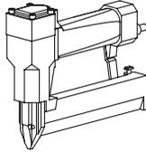
**Finishing nailer (for 18 gauge nails)**
