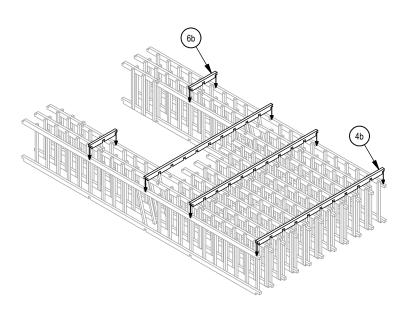
**STEP** Once spacer bars are properly placed. Start from the bottom of the rack, firmly apply pressure to lock in the joint. Then apply two
