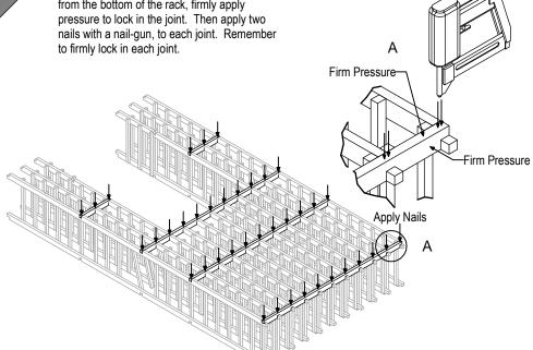
Place the middle ladders (2c) facing down on flat, soft surface, so not to damage front of racks. Space the ladders accordingly and put the back spacer bar (5b) into place. Make sure to center the spacer bar to the ladders. Spacer bar should extend past ladders at each end.
