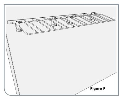
\*Alternate Installation\* Attaching to FCF-HD - Place the rack against the FCF-HD in the position where it is to be installed and ensure that it is horizontal using a level. To secure the rack, use the Self Drilling Screws provided with the FCF-HD and tasten the rack through each of the 8 mounting holes.
