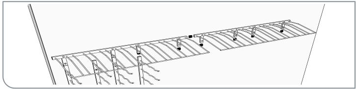
1. **Mark the mounting hole locations** - Position the rack on the wall where it is to be installed and use a level to ensure the rack is perfectly horizontal. Using a pencil, mark all 8 mounting hole locations (Figure A) and set the rack aside.
