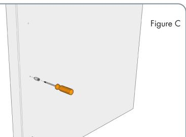
place through the bottom two mounting holes with the provided screws and fully tighten the toggle bolt.
