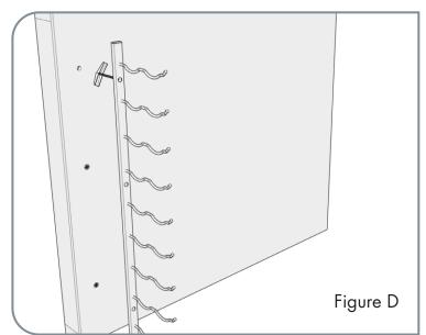
**7. Hang the second strip** — Repeat steps 3 through 6 with the second strip, centering it horizontally with the second mark on your wall from Step 1 and ensuring that the tops of the strips are even with each other.
