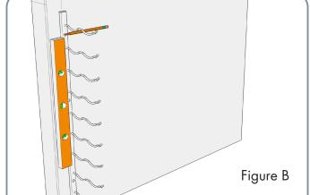
**2. Lay out the wall** — Starting at least  $2\frac{3}{4}$ " (70 mm) from adjacent wall or other obstructions, mark the centerline of the first strip. From there, measure  $7\frac{1}{2}$ " (190.5mm) from that mark for the distance between the neck and the base strips.
