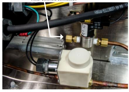
6. Locate the nearest water supply. Shut off water supply to the line and braze in a compression tee, or use a saddle valve adapter. Connect the water filter to the fitting and run ¼" copper from the filter thru the evaporator side opening and attach to the water solenoid inlet.
